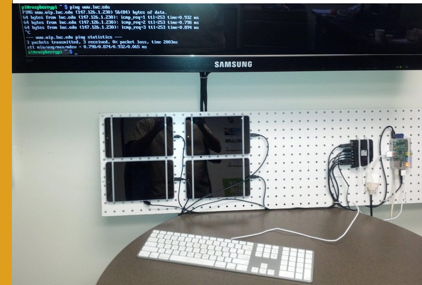
4x N7 Android Tablet Wall prototype with Raspberry Pi as server
